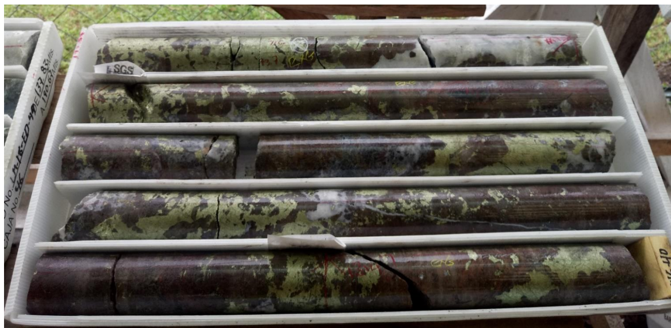
Figure 2 Hole LM - 18 - ED - 49: Semi - Massive Chalcopyrite in Magnetite
