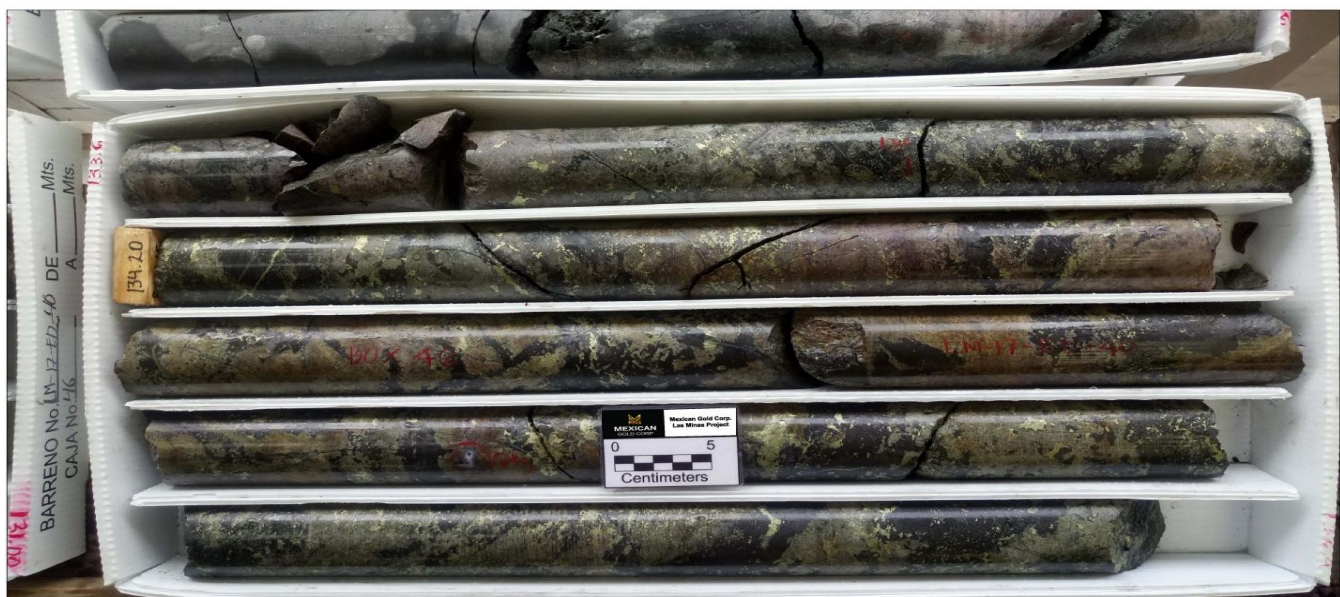
Figure 1: LM-17-ED-40 Example of Chalcopyrite Mineralization
